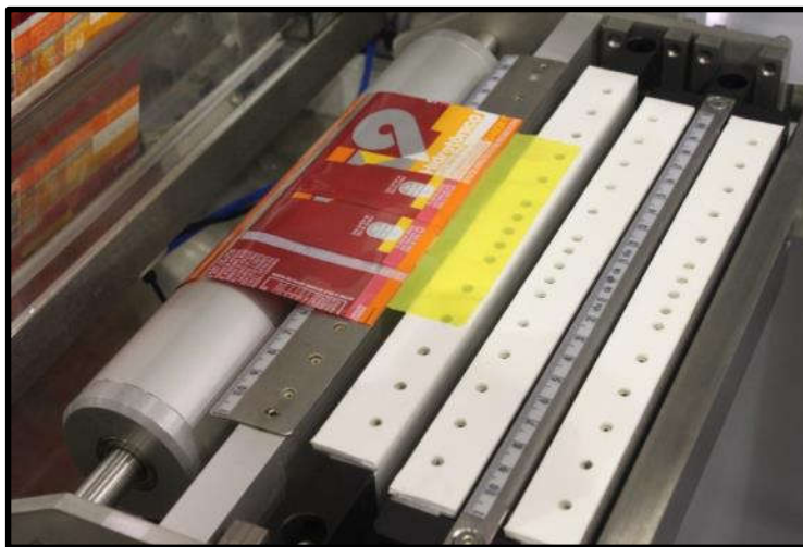
WEB ATTACHED TO TAPE AND PROPERLY ALIGNED
