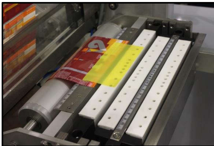
SPLICE TAPE IN POSITION – WEB UNDER TAPE
