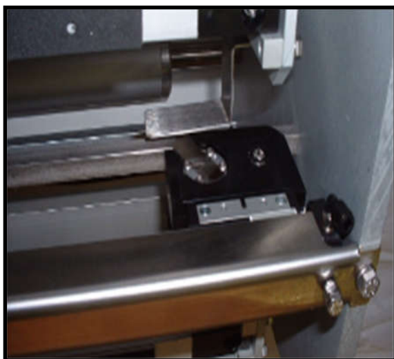
KNIFE HOLDER SHOWN AT ONE END OF TRAVEL PNEUMATIC CONNECTIONS AT EACH END OF KNIFE CYLINDER
