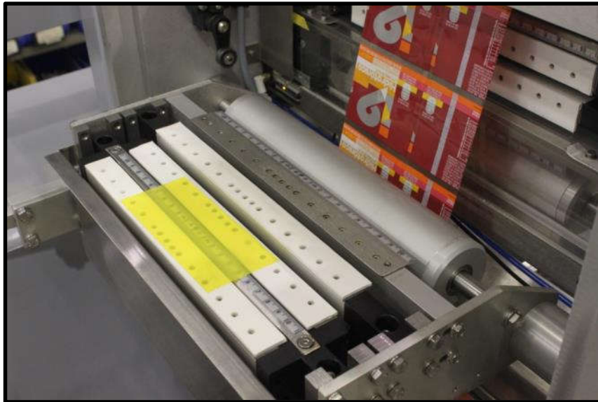
SECOND SIDE TAPE PREPARED ON RUNNING WEB SIDE OF HEAD
