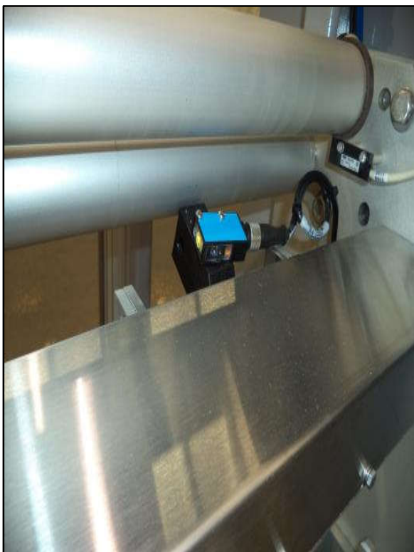
MAGNETIC WIF ENCODER ON UPPER GUIDE
