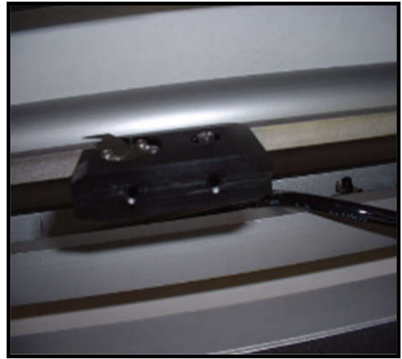
KNIFE HOLDER ON ANVIL/GUIDE INSIDE SPLICE HEAD
