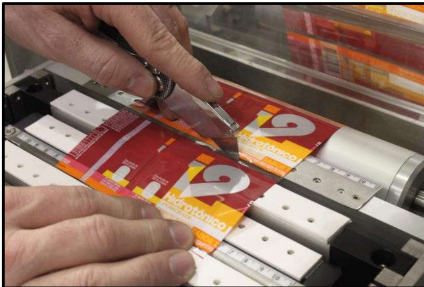
NEW WEB ALIGNMENT ON SPLICE HEAD AND CUT ALONG PREPARATION BAR
